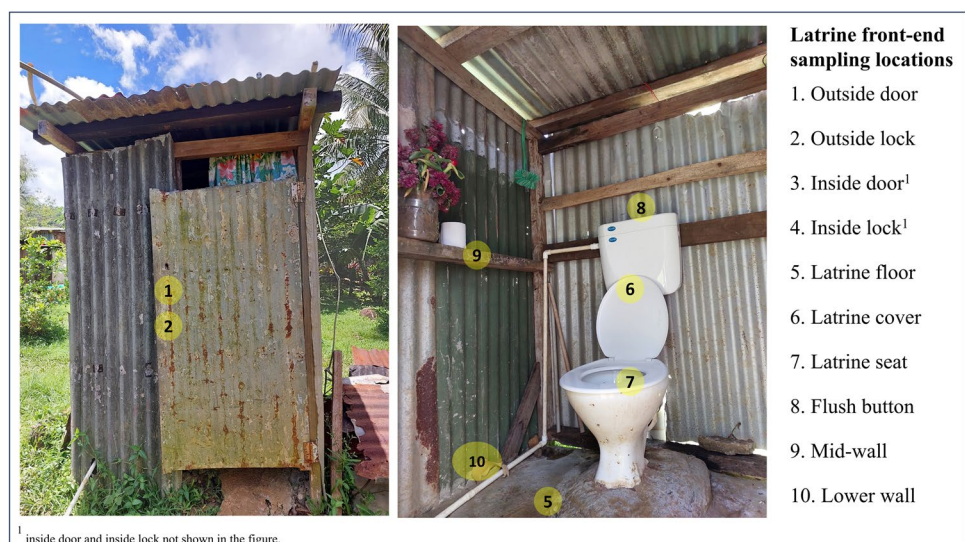
Fig. 2 In-depth front-end sampling locations of a cistern-flush latrine at Natadradave, Dawasamu, catchment. The yellow circles with numbers represent the sampling locations
