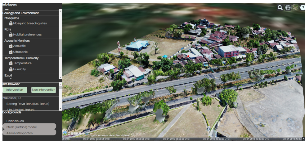
Fig. 2: Screenshot from platform prototype illustrating georeferenced, high resolution 3D mesh model overlaid into open-source satellite imagery
