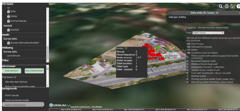
Fig. 3: Screenshot from platform prototype illustrating selection of a building to query household data on water, sanitation and hygiene factors
